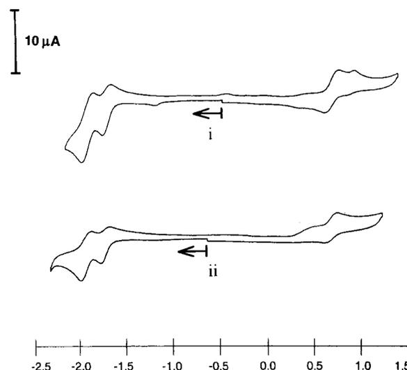
**Figure 4.** CV response of 1.0 mM solutions of the isomeric metallo dendrimers. (i) **17** and (ii) **16** in 0.1 M Et<sub>4</sub>N<sup>+</sup>TFB<sup>-</sup> in CH<sub>3</sub>CN at 298 K. Potentials are against internal ferrocene/ferrocenium. Scan rate: 200 mV/s.
