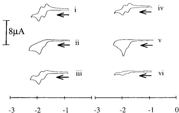
**Figure 5.** CV response of 1.0 mM solutions of dendrimers. (i) **34**, (ii) **35**, (iii) **36**, (iv) **31**, (v) **32**, (vi) **33** (the smaller current observed was due to the limited solubility of **33** that was presented in DMF) in 0.1 M Et<sub>4</sub>N<sup>+</sup>TfB<sup>-</sup> in DMF at 298 K. Potentials are against internal ferrocene/ferrocenium. Scan rate: 200 mV/s.
